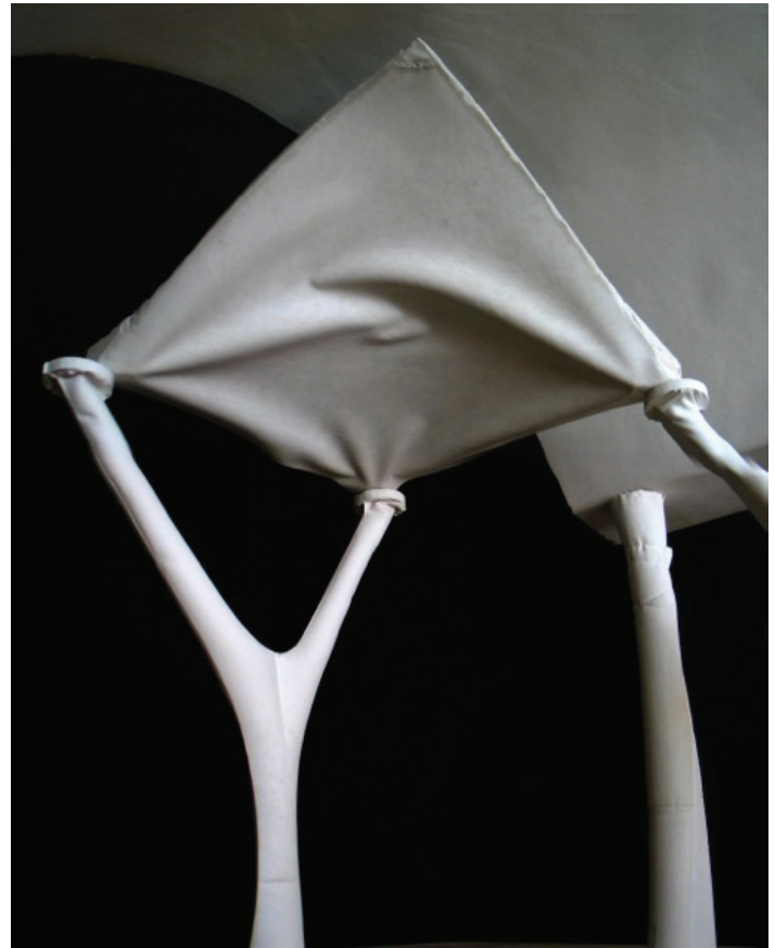
Figure 1. Examples of fabric formed columns and thin shell structures developed at CAST by Professor Mark West.
